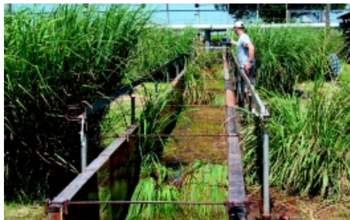
In a flume, grass hedges are tested at increasing water discharge rates until inundated and no longer effective.
