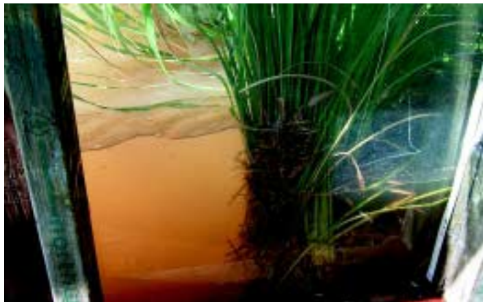
Windows in the flume’s side wall allow observation of flow patterns and effects of debris on the flow through the grass hedges.
